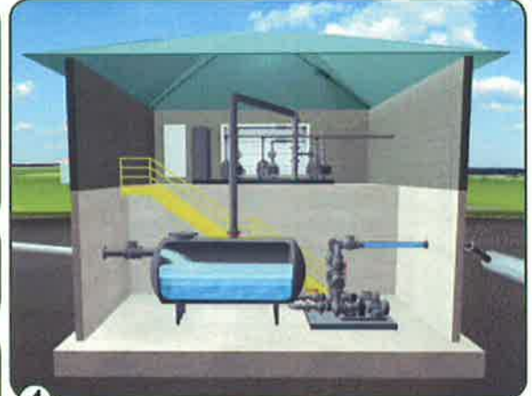
4 At the vacuum station, vacuum pumps cycle on and off as needed to maintain a constant level of vacuum on the entire collection system. Wastewater enters the collection tank. When the tank fills to a predetermined level, sewage pumps transfer the contents to the treatment plant via a force main.
