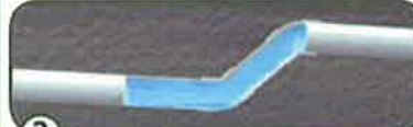
3 Wastewater travels at 15 to 18 fps in the vacuum main, which is laid in a sawtooth fashion to insure adequate vacuum levels at the end of each line.
