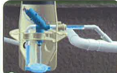
2 When 10 gallons of wastewater collects in the sump, the AIRVAC valve opens and differential pressure propels the contents into the vacuum main.
